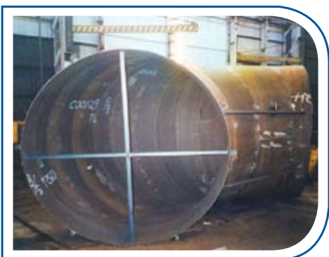
Vidaplate V34 cement meal duct
