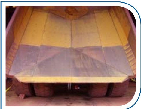
Truck bed lined with Vidaplate V37 and Bradken Q&T
