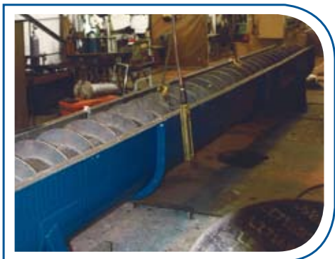
Screw feeder lined with Vidaplate V37
